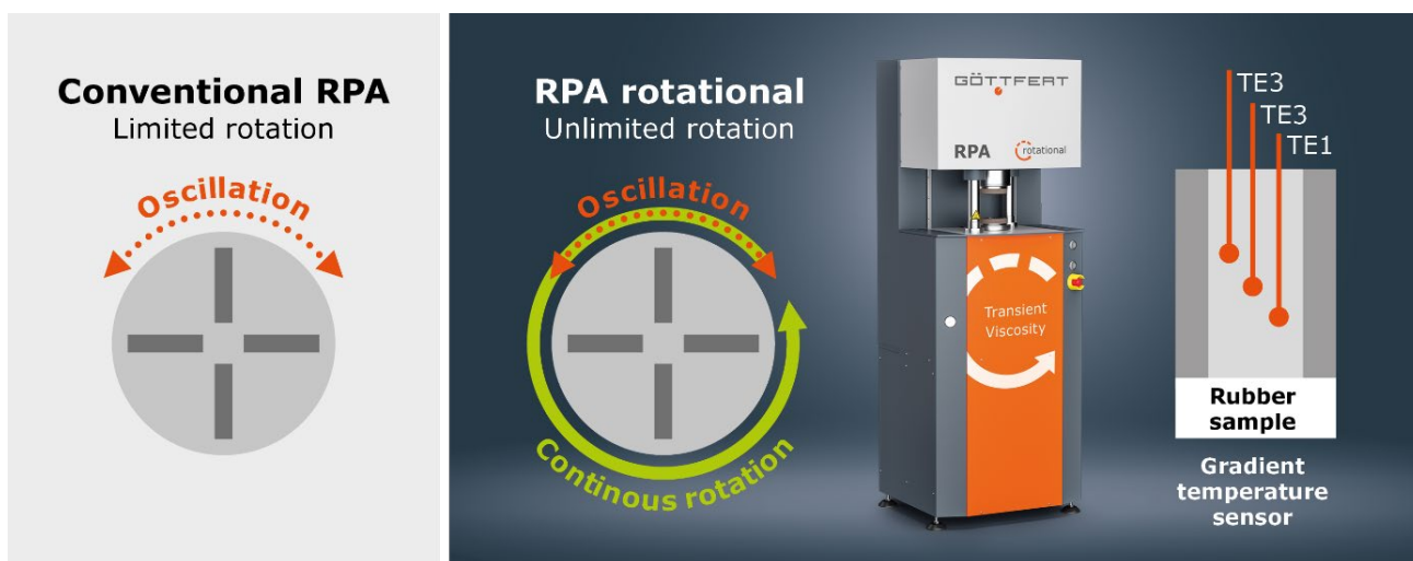
Figure 1: Conventional rubber process analyzers (RPA) are rotational rheometers with limited rotation (left side). Accordingly, measurements are mostly limited to oscillatory stimuli. The RPA rotational (right side) is one of the first RPAs with a moving die that can perform rotations of unlimited amplitude. This creates the possibility for continuous rotation measurements to determine the steady shear viscosity. Thanks to the built-in gradient temperature sensor, the temperature buildup due to dissipative heating can be detected and corrected, allowing for reliable viscosity data even under fast shear conditions. The figure is reprinted from a KGK Rubberpoint article 1 .
