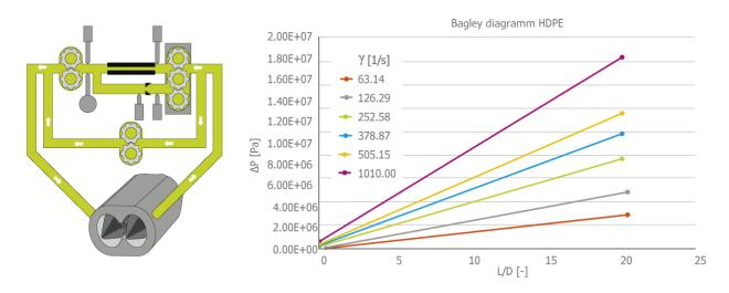
Figure 2: RTS with long and short die and Bagley Correction
