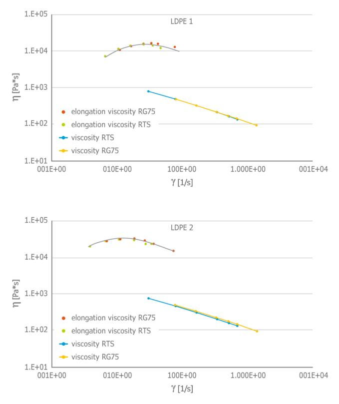
Figure 3: Comparison of shear and elongation viscosity between online and laboratory measurements of two LDPE
