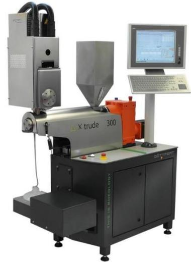
Fig. 1: ALR-R consisting of 1" lab extruder feeding RTS extruder
