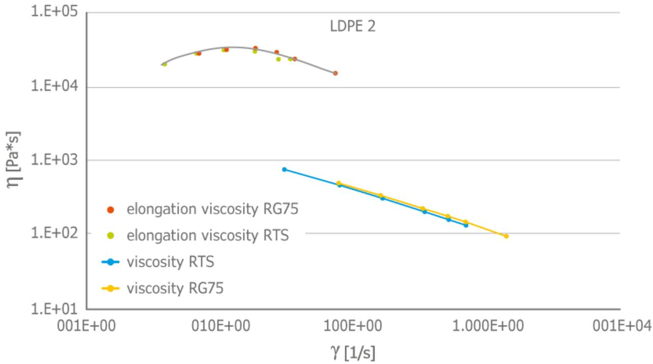
Figure 3: Comparison of shear and elongation viscosity between online and laboratory measurements of two LDPE
