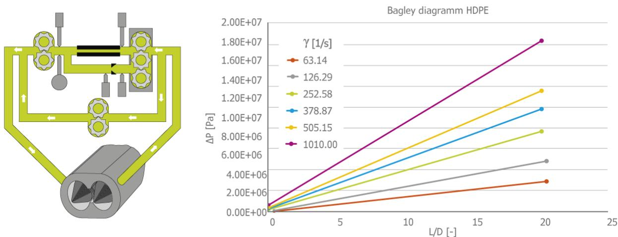
Figure 2: RTS with long and short die and Bagley Correction
