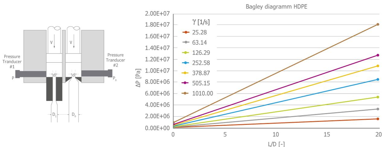
Figure 1: Twin Die capillary rheometer with Bagley correction
