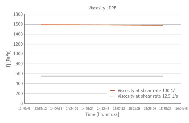
LDPE shear rate 100 1/s and 12.5 1/s of a 2 h run)
