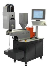
Fig. 1: ALR-R consisting of 1" lab extruder feeding RTS extruder
